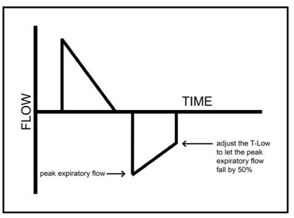
If oxygenation is the biggest problem, the  $T_{LOW}$  can be shortened to allow a drop in expiratory flow of 25%. This will result in less CO<sub>2</sub> being ventilated but will also keep some additional alveoli open and improve oxygenation.
