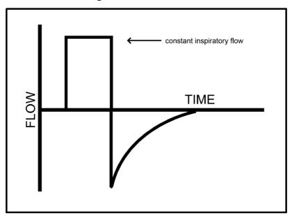
Constant flow is the pattern seen in older ventilators using volume control. When the ventilator gives a breath, it opens
