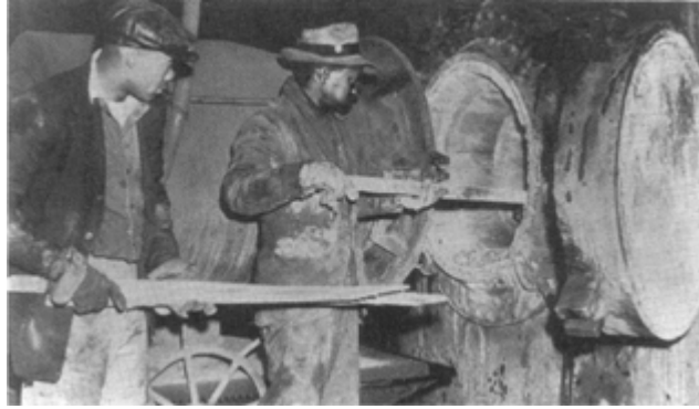
Sparrows Point workers cleaning a furnace by removing “slag,” a toxic by-product of molten metal, sometime in the 1940s. COURTESY OF THE DUNDALK-PATAPSKO NECK HISTORICAL SOCIETY
