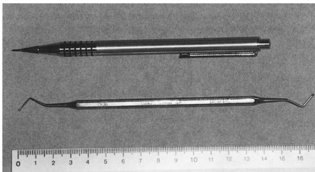
Fig. 6.1 Pressure probes: the telescopic pressure probe and the spherical filler used in dentistry.
