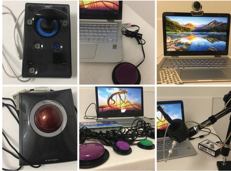
Figure 26-7 Examples of common navigation and selection methods, from left to right and top to bottom—Roller Joystick from Traxys, Swifty USB switch adapter, Orin Instruments and Jelly Bean switch, AbleNet Inc., TrackerPro head-controlled mouse from AbleNet Inc., SlimBlade trackball, Kensington, Mouse Mover/Hitch Computer Switch Interface from Able26Net Inc., Jelly Bean and Specs Switches from AbleNet Inc., and Jouse 3 from Compusult Limited.
