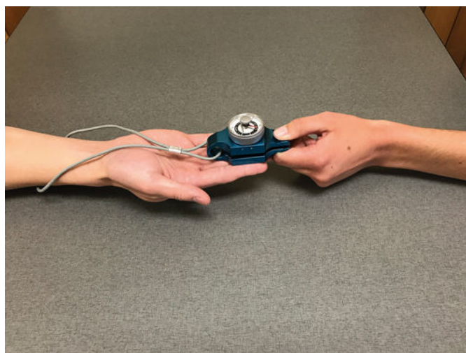
Figure 13-140 Measuring lateral pinch strength with a pinch gauge.
