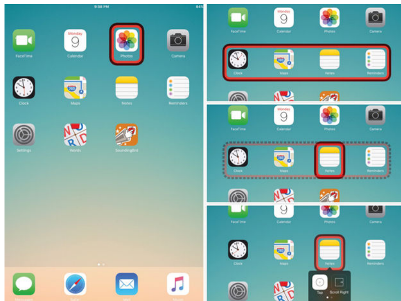
Figure 26-4 Row-column 1-switch scanning on an iPad platform.
