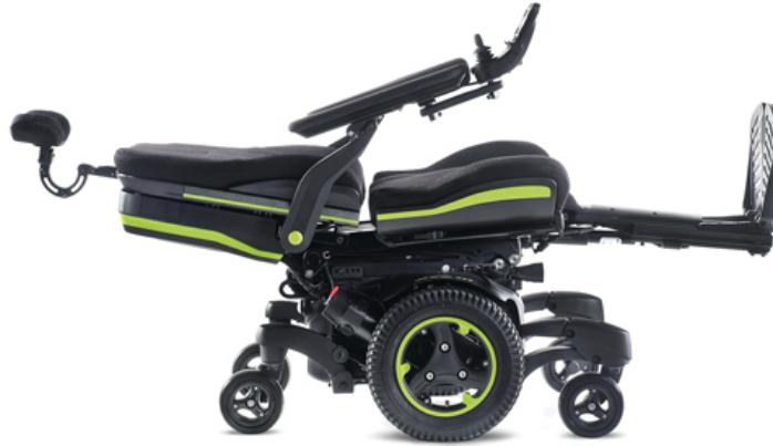
Figure 25-9 Recline with elevating legrests on a power wheelchair. (© Sunrise Medical.)
