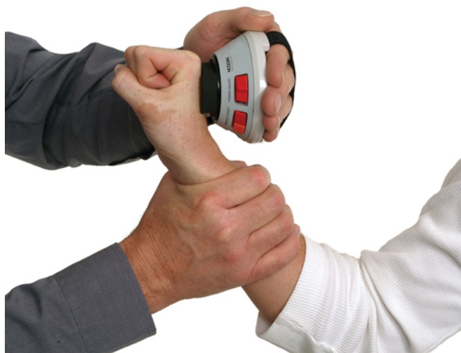
Figure 13-137 Example of handheld dynamometer for isometric strength testing. (Picture courtesy of Hoggan Scientific.)
