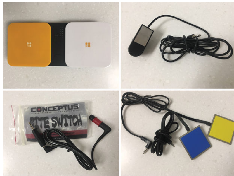
Figure 26-3 Switches with various characteristics. Examples of switches top to bottom, left to right (wireless) Blue2 (AbleNet Inc.); (wired) Micro Light (AbleNet Inc.), Bite Switch (Conceptus), Pal Pad (Adaptation).
