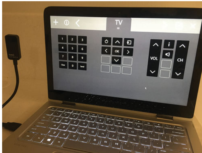
Figure 26-11 EyeR (TobiiDynavox) USB dongle with infrared emitter pair with the Virtual Remote computer software to create a computer-based electronic aids to daily living (EADL).
