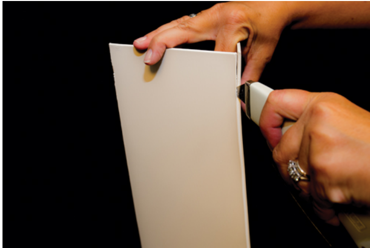
Figure 23-15 Cutting thermoplastic material with a utility knife.
