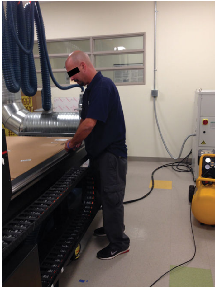
Figure 21-11 Standing workstation. Worker standing at a laser machine. Note flexion of neck and extension of elbows resulting from low height of working surface. Worker would benefit from an ergonomic mat for prolonged standing.
