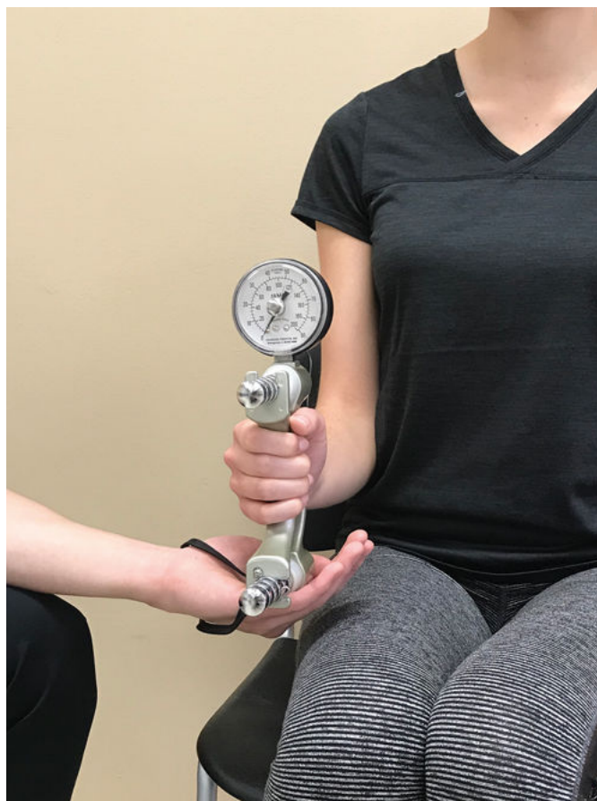
Figure 13-138 Measuring grip using a dynamometer. The client's upper arm is close to his body, and the elbow is flexed to 90°.
