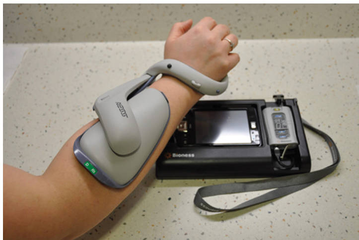
Figure 22-44 Ness H200—Device uses a low-level electrical stimulation to activate weak or paralyzed muscles within the forearm to improve hand function.
