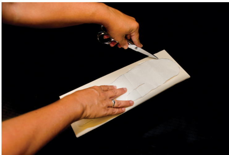
Figure 23-16 Scoring heated material with scissors to outline pattern.
