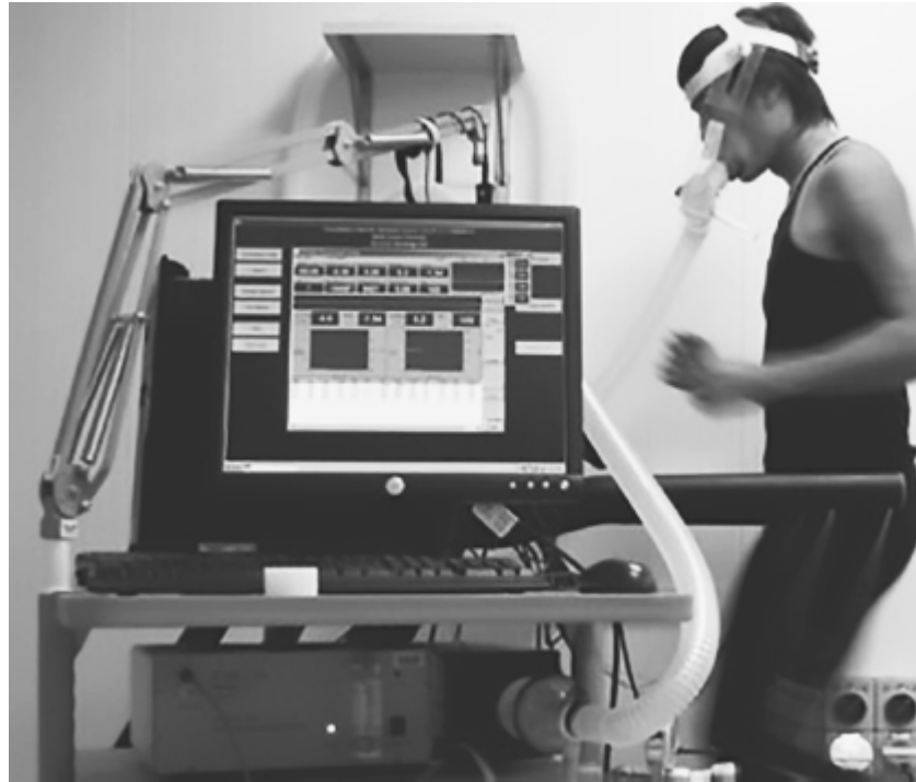
Figure 2.4. Indirect calorimetry using a mouthpiece connected to a metabolic cart
