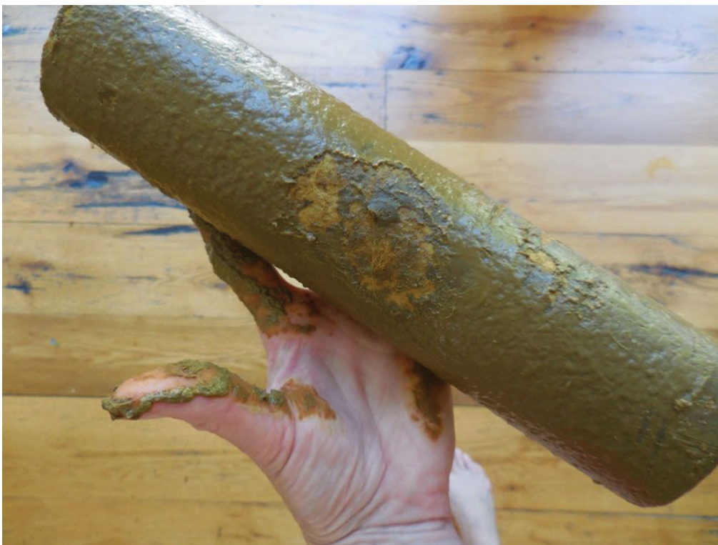
Figure 5.4 Image of author’s own old RO filter during replacement (taken by author AC, fall of 2018).
