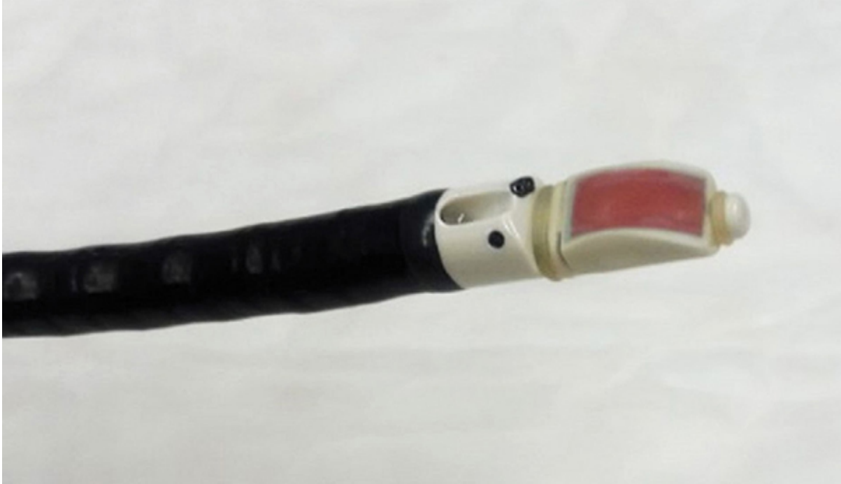
Figure 11-19. Distal end of a curvilinear endobronchial ultrasound scope showing the ultrasound transducer.
