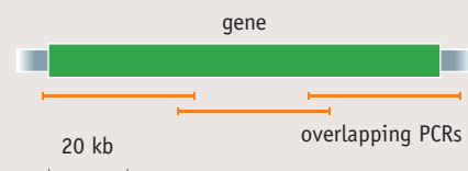
FIGURE 3 Amplification of a gene of approximately 100 kb as a series of overlapping PCRs.
