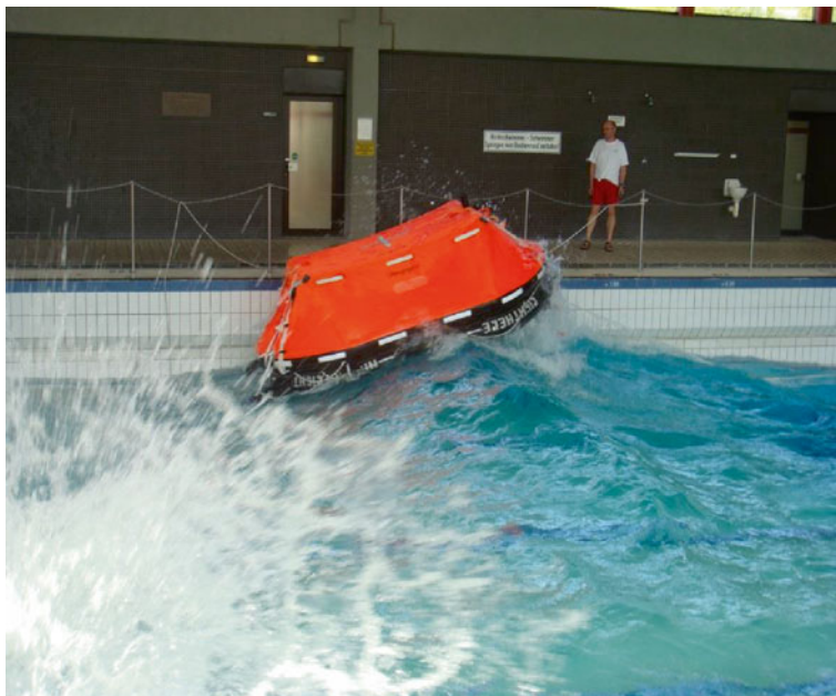
Fig. 10.5 Inflatable life raft exposed to one-meter-high waves
