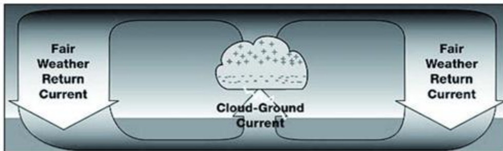
Figure B-1. Global electrical circuit. A current coming up from the ground at the location of lightning (depositing electrons into the earth) and returning to the ground elsewhere.
