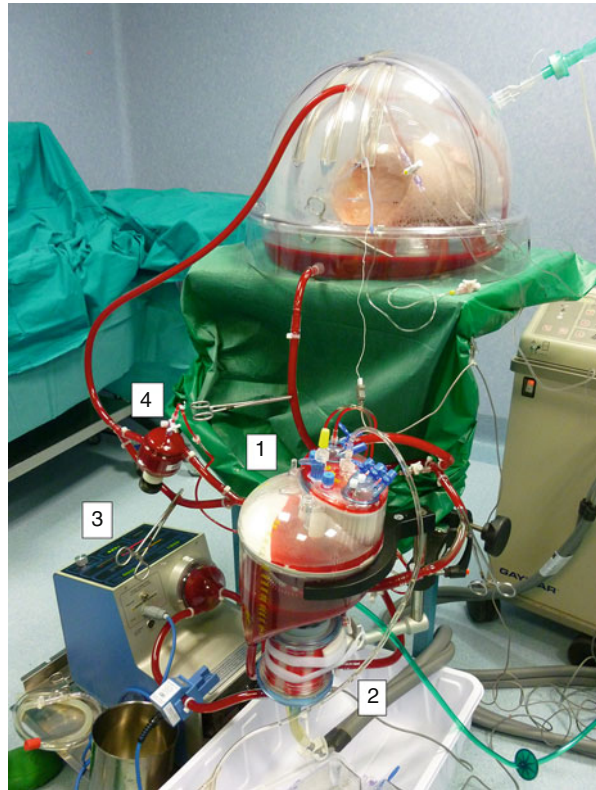
Fig. 29.1 Figure shows the circuit used to perfuse the isolated lungs. It consists of a blood reservoir (1) connected to a gas oxygenator with a built-in heat exchanger (2), a centrifugal pump (3), a leukocyte arterial filter (4), and a non-heparin-coated polyvinyl tubing
