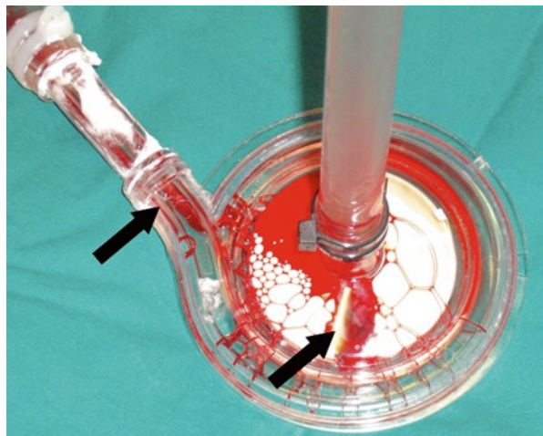
Fig. 35.2 Black arrows showing clots in the pump head after a circuit change-out
